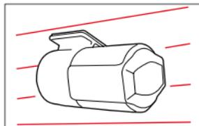
Remove the protective tape and attach the rear camera in proper location in windshield.
