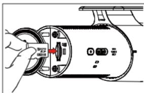
1. Insert the MicroSD card in the card slot. (Check the MicroSD card direction)
