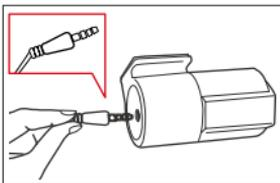
Connect the ( — ) shape's rear camera cable to a rear camera connection and the ( ㄣ ) shape's one to the body.
