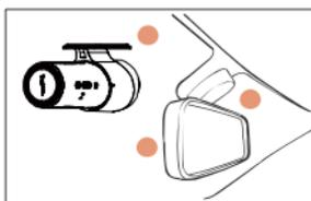
4. Attach the product in place on the top of front windshield or middle, left or right of the mirror.
